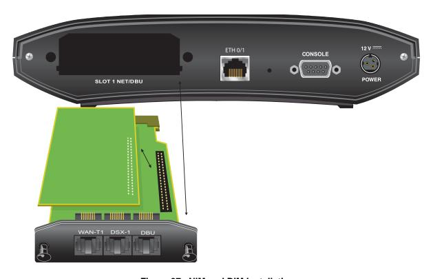
Figure 37. NIM and DIM Installation
